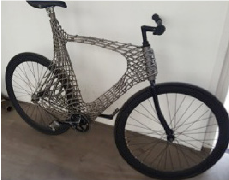
A bike frame manufactured in 3D printing by robots by MX3D.
