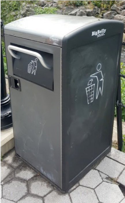
The smart waste bin equipped with solar powered sensor that senses how full the bin is and send a signal to service provider via Wi-Fi.
